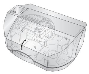
• The Publisher will automatically position the cartridge carrier and Robotic Arm to allow for easy access to the bin.
