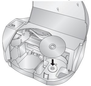
• Load the Input Bin (the bin located on the right-hand side of the Publisher) with up to 20 blank discs.
