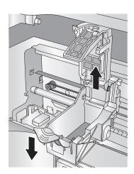
3. Remove the ink cartridge from its packaging. Slowly remove the tape covering the cartridge's print head.
