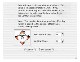
Look at the finished alignment disc and pick the numbers that come closest to lining up with one another. For instance, on the disc shown in this manual, the vertical alignment is 2 and the horizontal alignment is 0. Enter this in the alignment dialog box.
