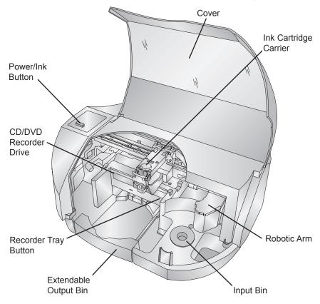
The **Robotic Arm** moves discs from the Input Bin, to a CD/DVD Recorder, to the printer, and finally to the Output Bin.
