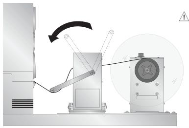
**Important!** To minimize the slack loop that will be created under the rewinder, it is very important that you engage this lever immediately after the label stock is taped to the core.
