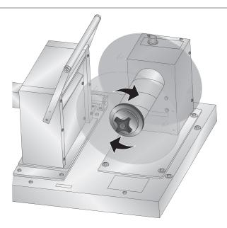
**Note:** Some cores may be shorter than the stock width. If so, make sure the distance between the label guide discs is slightly larger than the stock width.
