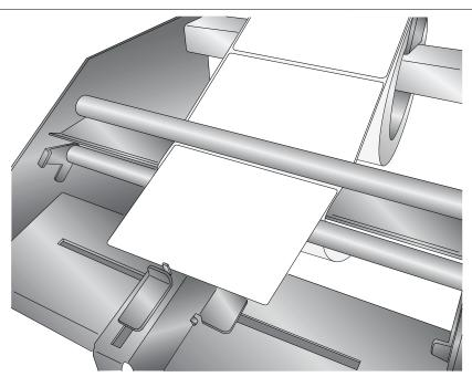
4. Pull the label off the liner with a quick upward motion. (Figure 3-4.)
