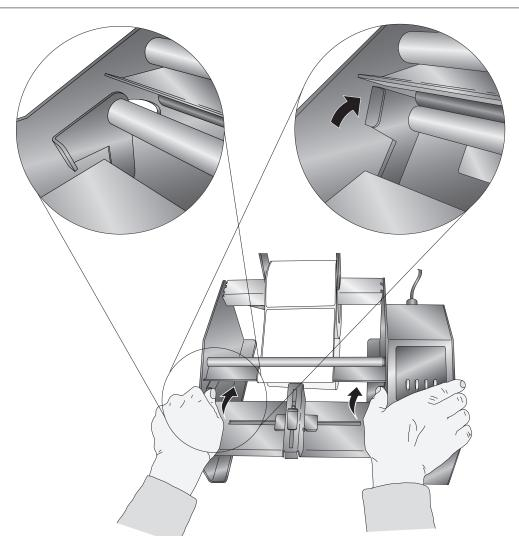
11. Move the Label Sensor Bracket where desired within the width of the label. (Figure 2-9.)
