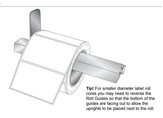
Place the Roll Drag Arm under the Roll Bar. The Roll Drag Arm may be placed on either side of the Roll Bar, but the rounded tip of the Roll Drag Arm should be located in the center of the inside of the core. The arm is spring loaded so that there is downward pressure on the inside of the roll. This helps prevent application alignment problems near the end of a roll. (Figure 2-3.)
