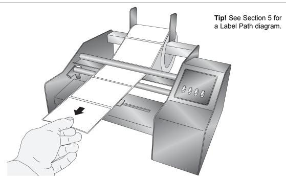
8. Take the loose label stock and feed it between the Liner Idler Roller and the Liner Drive Roller. (Figure 2-6.) In order to feed the label stock between the rollers, the Liner Idler Roller should be in the unclamped position. (See Figure 2-10 for a detailed diagram of the Liner Idler Roller positions.)
