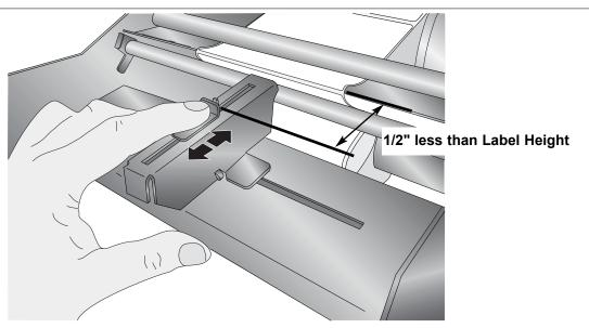
For example, for a 4" wide x 2" high (101.6mm x 50.8mm) label you would set this distance to approximately 1-1/2" (38.1 mm). The exact distance is not critical. It is only important that you set the distance so that the label does not come off the liner when presented. If the label height dictates the sensor be moved beyond the available travel, set the sensor to the minimum or maximum position as applicable.
