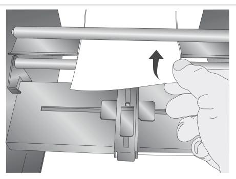
**Note:** For labels higher than 3" (76.2 mm) you will have to slowly pull up on the label with continuous force until the end of the label clears the Guide Roller. For these type of labels set the label sensor bar to the maximum distance from the Peel Edge.
