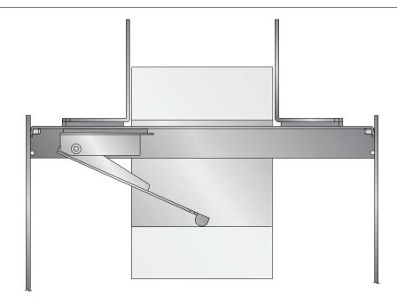
Place the removed Roll Guide back on the Roll Bar and slide it close to, but not touching the label stock roll. (Figure 2-4.)
