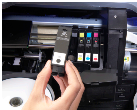
The 4100 OEM Print Engine utilizes large, separate CMYK ink cartridges.
