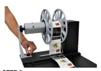
**STEP 6** Install the support and fasten it to the base through the knob.
