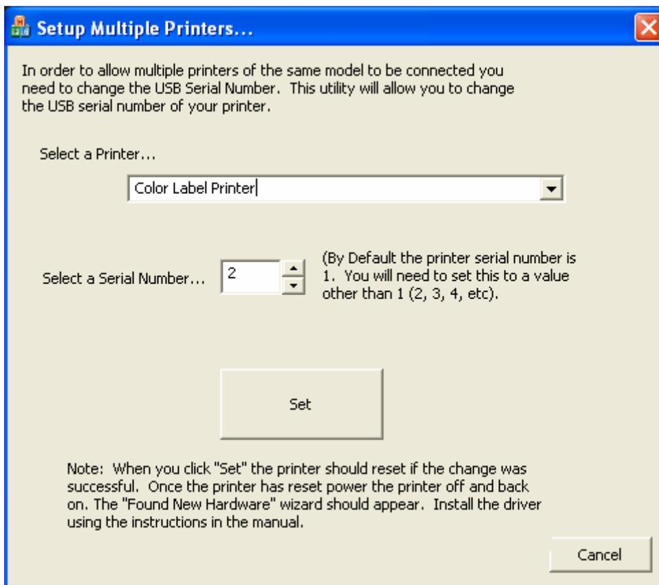
**C. Installing the Second Driver.** To install the second driver, unplug the power cable from the printer, wait a few moments and then plug the power cable back in. A found new hardware wizard will appear. Follow through the wizard to install the printer driver.
