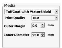
you select a media type from this box the Print Quality, Outer Margin and Inner Diameter are automatically adjusted to fit that media.
