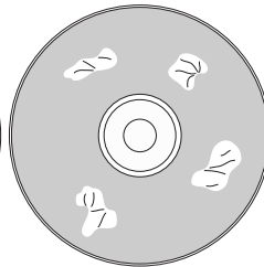
Uneven coverage due to inadequate heat
