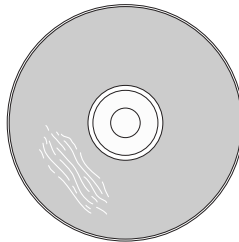
Wrinkle in film caused by excessive heat
