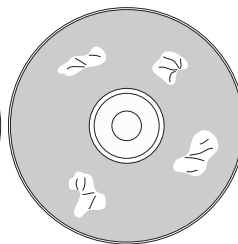
Uneven coverage due to inadequate heat
