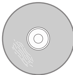
Wrinkle in film caused by excessive heat
