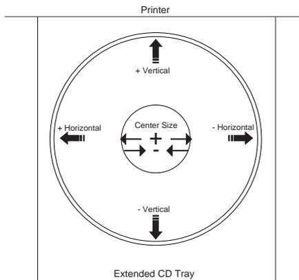
**HINT:** Notice the direction the **Vertical** and **Horizontal** adjustment arrows point within the Calibration window are representative of the direction the printed image moves on the CD-R.
