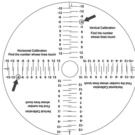
5. Along the Vertical axis of the printed CD template, find the number whose lines touch. For example, in the above illustration, the number would be -6. Enter that number into the Vertical box of the Calibration window. Repeat this same step for the Horizontal axis.
