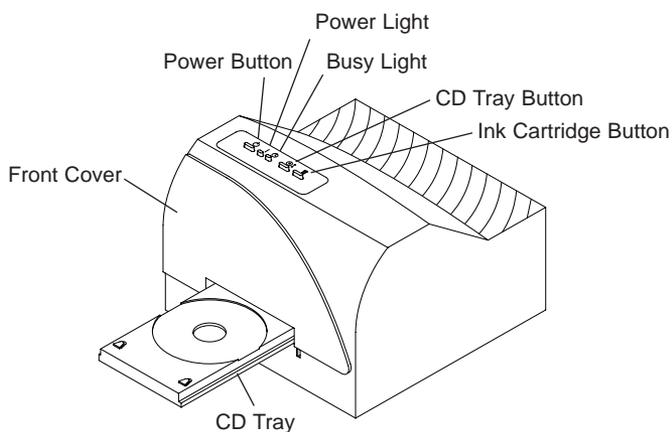
The **⏻ Power Button** turns the printer's power ON and OFF. This button also serves to cancel the current print job if a print error occurs and to reset the printer for the next print job.
