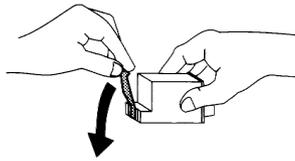
3. If switching between color and monochrome cartridges, simply remove the extra cartridge from the Spare Ink Cartridge Holder by grasping the top of the cartridge and firmly pulling it straight toward you. You will hear the cartridge snap out of position.
