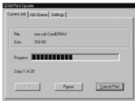
The **Current Job** tab tells you the name and size of the file printing, the progress of the overall print job, as well as the total number of copies left to print. It also provides buttons which allow you to pause or cancel the print job at any time during the printing process.
