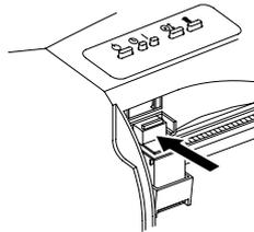
7. Press and release the
