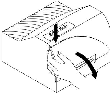
2. If installing a new, replacement ink cartridge, remove the cartridge from its packaging and remove the tape covering the cartridge's printhead. **DO NOT TOUCH THE COPPER AREA!**
