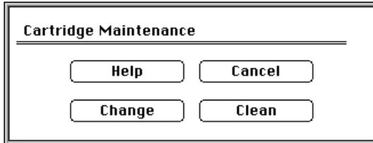
Select the **Change** button to move the printer's ink cartridge carrier to the load position in order to change ink cartridges. Note that pressing the printer's **Ink Cartridge** button serves this same purpose. See Section 2 for further information on changing ink cartridges.
