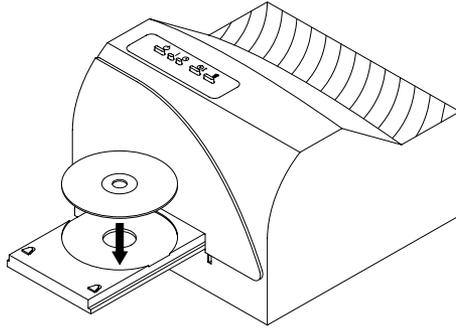
1. With the printer's front cover shut, press and release the
