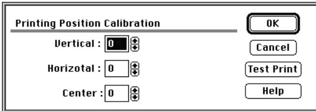
When facing the printer, the **Vertical** adjustment moves the printed image toward the printer if a positive number is entered and away from the printer if a negative number is entered. The **Horizontal** adjustment moves the printed image toward the left-hand side if a positive number is entered and toward the right-hand side if a negative number is entered.
