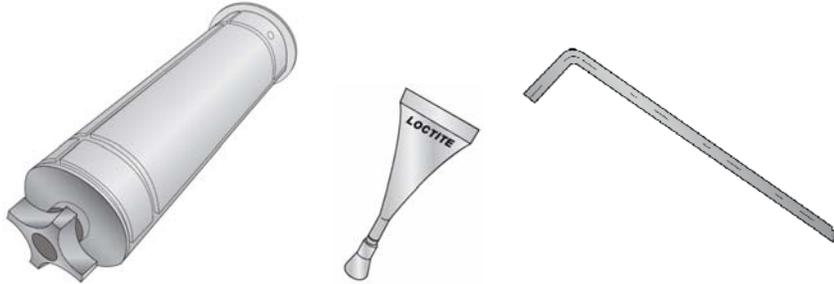
5. Partially remove the two set screws on the mandrel so that approximately ½ inch (1 cm) is exposed. Crack the top off the Loctite container and place two drops on each set screw. Reset each screw until it is flush with the outside of the mandrel. Attach the mandrel to the unwinder (left side) drive shaft. Line up the holes in the chuck with the flat edges on the drive shaft. The holes must correspond with the flats or the set screws will not hold the chuck in place.
