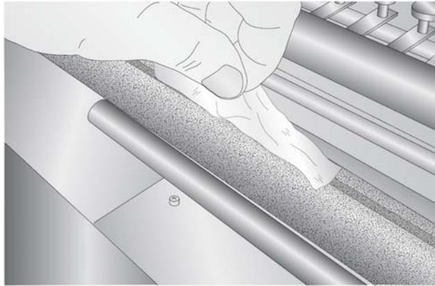
3. Push the foam together along the entire length of the slit in the foam roller. The adhesive will hold it together.
