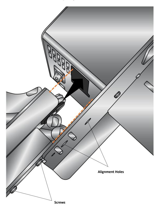
4. Align the screws on the side of the arm with the holes in the labeler frame.
