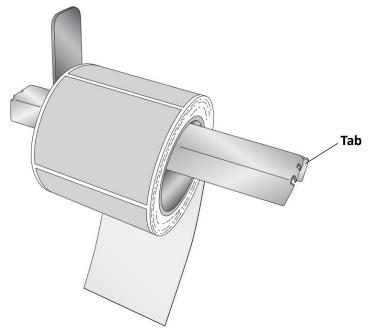
**Tip!** For narrower label roll cores (less than 3.625 in. [92 mm]) you may need to reverse the roll guides so that the bottom of the guides are facing out to allow the uprights to be placed next to the roll.
