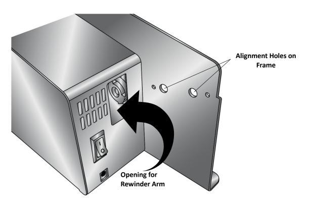
3. Insert the rewinder arm into the opening as shown.
