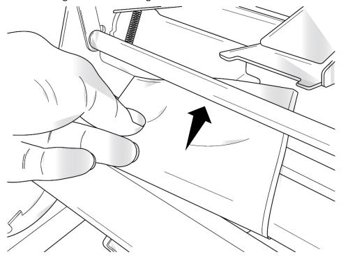
12. Pull the label stock all the way through until the end of the roll is lying over the top of the label stock roll. Adjust the label stock forward or backward so that the peel edge is between two labels.
