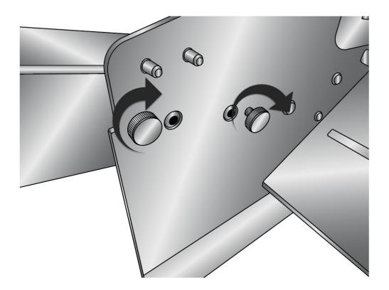
6. If not already attached to the rewinder arm, the liner guides must be installed on the rewinder. Locate the liner guides. Slide one of the label guides onto the shaft with the black cylinder facing you. Note that the holes in the cylinder must align with the flats on the shaft.
