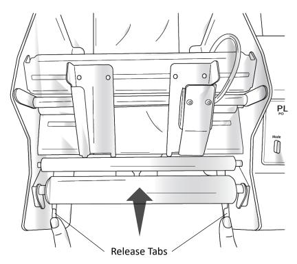
17. Adjust the label guides so that they are almost touching the edges of the label stock. Do not pinch the labels between the guides. If the guides are loose, pull them away from the label stock, and tighten the thumbscrews. When the thumbscrews are tight, move them into place on either side of the the label stock.
