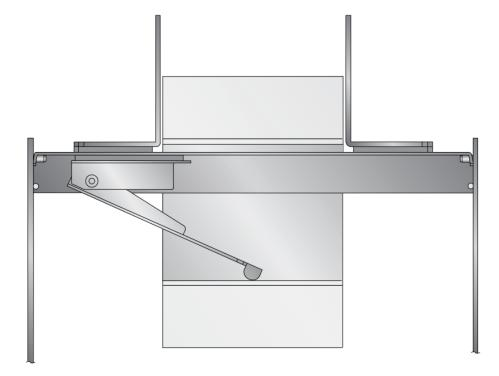
5. Place the removed roll guide back on the roll bar and slide it close to, but not touching, the label stock roll.
