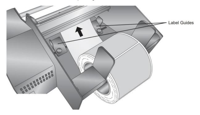
8. To make it easier to feed the label stock, first pull out the pouch idler roller until it locks into a open position. There will be approximately one inch of space between the pouch drive roller and the pouch idler roller.
