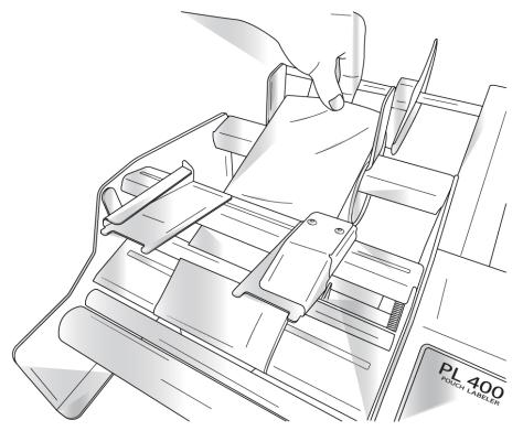
13. If necessary, adjust the position of the liner on the peel edge left/right to align the liner with the label stock roll. Also, adjust the label sensor using the label sensor bracket so that the label sensor flag is roughly centered on the label stock.
