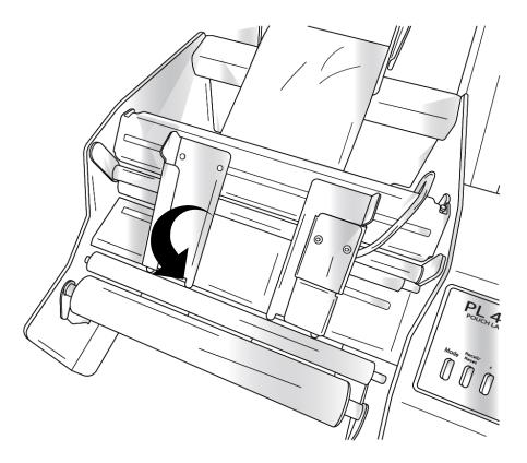
16. Push down on the release tabs on either side of the labeler simultaneously to release the pouch idler roller back to its clamped position.
