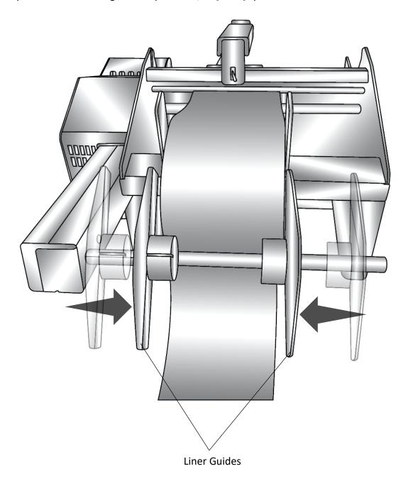
19. Fold the leading edge of the liner and hook the folded edge around the tabs on each liner guide. You may need to label a few pouches to have enough liner to hook the fold on the tabs. See the next section. **Tip!** We recommend trimming the liner to length with scissors to minimize the resulting slack in the liner and to provide a square leading edge to fold.
