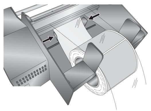
18. Begin applying labels until you have enough liner to reach the liner rewinder. Set the position of the liner guides to provide 1/8" [3mm] space on each side of the liner.
