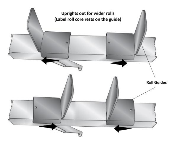
Uprights in for narrow rolls (Label roll core rests on the bar)
