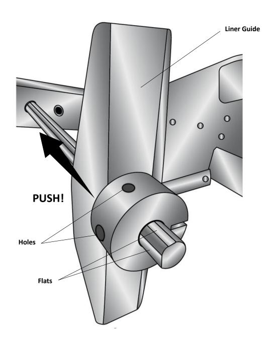
7. Push the remaining liner guide onto the shaft with the black cylinder facing away from you. The guides should be calibrated from the factory to stay in place during Label application, but allow adjustment of their position without the use of tools. If more or less sliding force is desired, the set screws in the black cylinders can be tightened or loosened with a 2mm hex key provided. The two set screws in each cylinder should be tightened equally.
