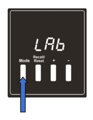
Press for 5 seconds and then press two more times until Lab is displayed
