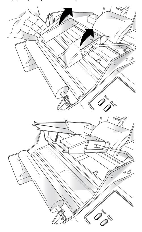
10. Pull approximately 12 inches [30 cm] of label stock out beyond the peel edge OVER the pouch idler roller. *Remove the labels from this section of the label stock! You may still apply these labels by hand.* You may wish to engage the label load mode discussed in Section 5D to assist with feeding label stock through the labeler for this step and the next step.
