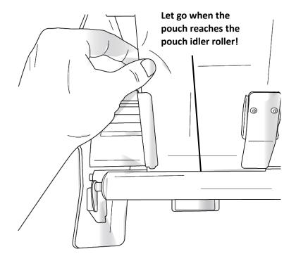
Important Note: Do not push or hold the pouch when the labeler is feeding the pouch.
