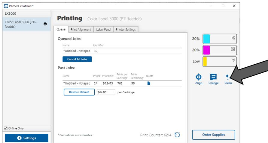
2. Determine if printing is now acceptable by printing your image. If the sample has missing colors or voids within a color strip, remove the cartridge from the printer and proceed to step 4.
