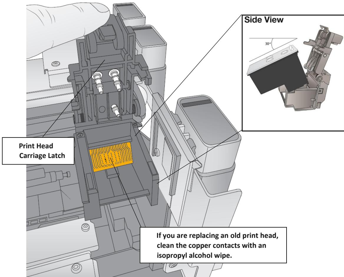
7. Press down firmly near the back of the print head to ensure good contact and proper alignment when you close the lid.
