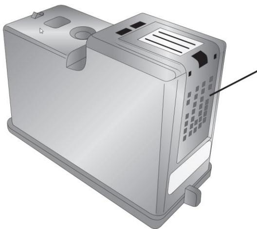
Dry excess water from cartridge. Ensure cartridge contacts are completely dry. Printer damage may result if cartridge contacts are not completely dry.
