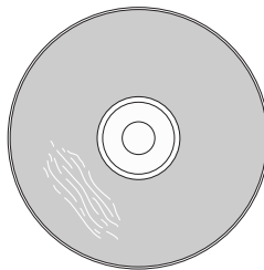
Wrinkle in film caused by excessive heat
