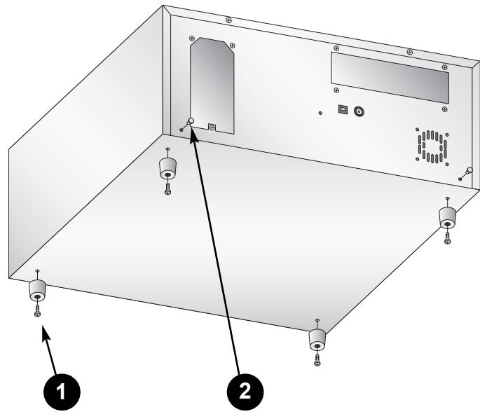
3. Place unit in Rackmount Bracket and secure to the back of unit using provided Phillips screws.
