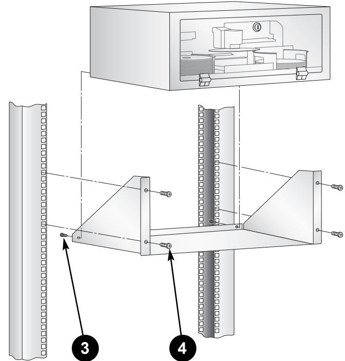
4. Secure Rackmount Bracket and unit to Rack using 4 screws provided with the Rack.
