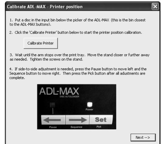
You can recalibrate at any time by opening Primo DVD - Click the robotics menu - select options - Click the **Calibrate ADL-MAX** button. If you are using RoboPrint, click **Robot Options - Calibrate ADL-MAX**.
