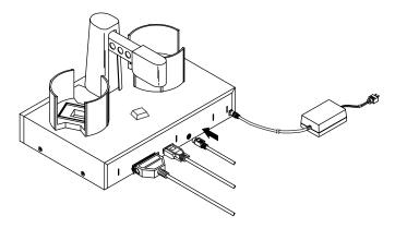
Attach the optional printer stand (required for a printer installation) to the Duplicator by locating the connecting tabs and inserting them into the slots on the rear panel of the Duplicator. For the Ink-Jet CD Printer, the stand is attached in the center of the Duplicator.
