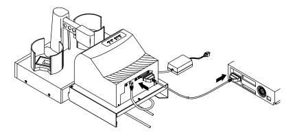
11. Make sure that all cables are routed neatly underneath and out the back of the printer stand and that no cables are underneath the Duplicator or printer stand feet.
