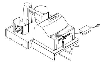
10. Connect the printer with an IEEE 1284 compliant parallel cable. One end is connected to the parallel port on the rear panel of the printer. The other end is connected to the parallel port of your PC. Make sure that your PC's parallel port is set to ECP mode. If you don't know how to check this or how to change it, refer to set-up section of the printer's Operator's Manual.
