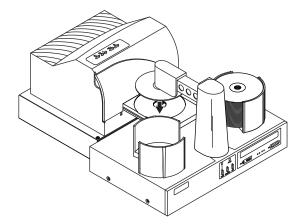
After printing, the printer's CD Tray opens automatically and the Robotic Arm picks the CD and transports it to the Output Bin. The process starts over and repeats until all blank discs are gone or the number you have specified via software are copied and printed.
