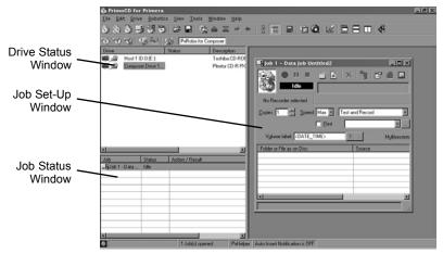
Under this window there are several adjustable-size windows that indicate what you've setup and what's happening: the Drive Status Window, the Job Status Window, and the Job Setup Window. A sub-Window called the Activity Log is also available, but it is hidden upon initial boot-up of the software. Here's a short explanation of each Window:
