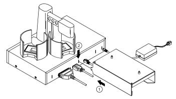
For either printer, find the locating holes on the bottom plate of the printer.
