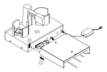
For the Thermal CD Printer, the printer is mounted on the left side of the Duplicator.
