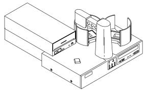
Note that the Thermal CD Printer attaches to the left side of the printer and that the Output Bin is located in a different spot due to the location of the Thermal CD Printer. When you first power-up the Duplicator, it will automatically do a search for where the Input and Output Bins are located and from then on will know where to pick and place discs.
