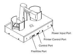
The FireWire (IEEE 1394) Port of the duplicator is for connection to your PCs internal FireWire board.
