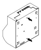
Position the printer on the stand so that the printer stand locating pins are inserted into the locating holes of the printer.
