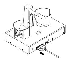
4. Connect the Serial Interface cable. One end is connected to the DB9 connector on the rear panel of the Duplicator. The other end is connected to your PC's DB9 COM1 port. If COM1 is already used for another device, you can use COM2 or COM3 and follow on-screen instructions later in the set-up procedure for changing the default serial port for the Duplicator.
