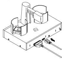
5. Apply power to the Duplicator. One end of the power adapter's cord is attached to the power input port on the rear panel of the Duplicator. The other end is connected to a suitable wall outlet. Use of a high quality, commercially available surge suppressor is highly recommended.
