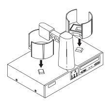
b. Put a stack of blank CDs in the Input Bin (the one on the right side).
