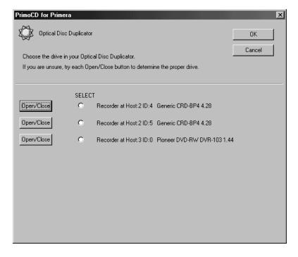
This dialogue box will allow Prassi to identify the drive in your Duplicator. Each recording drive installed on your system will be listed in this dialogue box. Click each **Open/Close** button to ope the recorder drive, then click the appropriate **SELECT** radio button for the drive installed in your Duplicator.
