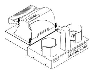
Check one more time for printer alignment after the screws have been tightened down, just in case something changed while you were making the adjustment. Re-align if necessary.
