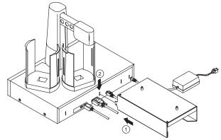
For either printer, find the locating holes on the bottom plate of the printer.
