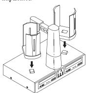
b. Put a stack of blank CDs in the Input Bin (the one on the right side).
