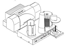
5. Through software control, you can perform a verification test on each CD-R disc before recording. If a disc does not pass (meaning that all or part of that disc is not recordable), the Robotic Arm picks it out of the CD Tray and sends it to the Reject Area, located at the front left side of the Duplicator. Rejected discs simply drop off of the front of the unit.
