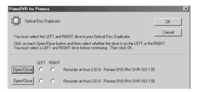
This is necessary for PrimoDVD to identify the drives. All recording drives installed on your PC will be listed in this dialogue box. Click the Open/Close button to see whether the left or right drive opens, then click the corresponding radio button. Proper automated robotic movements require you to select the right drive and left drive correctly!
