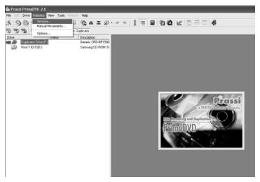
4. Click on Check Communications. You will get a dialog box saying "Communication OK. System Idle." If you don't, check that all cables are connected securely. Or, change the serial cable from COM1 on your PC to COM2 or COM3 and change the setting in the Control Port drop down menu. Try again until you get the "Communication OK" message.
