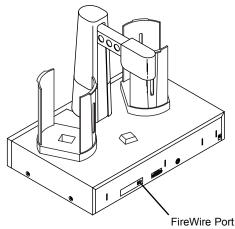
The FireWire (IEEE 1394) Port is for connection to your PC's internal FireWire card.
