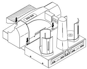
Check one more time for printer alignment by pressing after the screws have been tightened down, just in case something changed while you were making the adjustment. Re-align if necessary.
