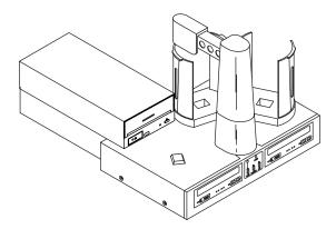
Note that the Thermal CD Printer attaches to the left side of the printer and that the Output Bin is located in a different spot due to the location of the Thermal CD Printer. When you first power-up the Duplicator, it will automatically do a search for where the Input and Output Bins are located and from then on will know where to pick and place discs.
