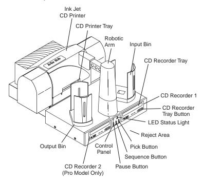
**CD Recorder 1** is the first drive the Duplicator loads and unloads as discs are copied
