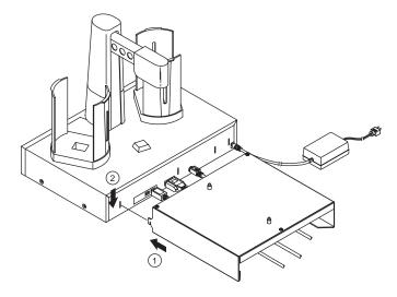
For the Thermal CD Printer, the printer is mounted on the left side of the Duplicator.
