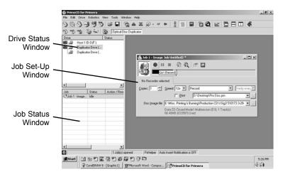
Under this window there are several adjustable-size windows that indicate what you've set-up and what's happening: the Drive Status Window, the Job Status Window, and the Job Setup Window. A sub-Window called the Activity Log is also available, but it is hidden upon initial boot-up of the software.
