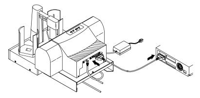
11. Make sure that all cables are routed neatly underneath and out the back of the printer stand and that no cables are underneath the Duplicator or printer stand feet.
