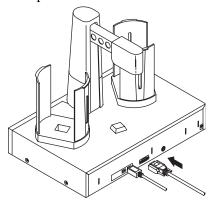
5. Apply power to the Duplicator. One end of the power adapter's cord is attached to the power input port on the rear panel of the Duplicator. The other end is connected to a suitable wall outlet. Use of a high quality, commercially available surge suppressor is highly recommended.
