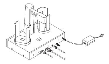
8. Attach the optional printer stand (required for a printer installation) to the Duplicator by locating the connecting tabs and inserting them into the slots on the rear panel of the Duplicator. For the Ink-Jet CD Printer, the stand is attached so that it is on the left side of the Duplicator.
