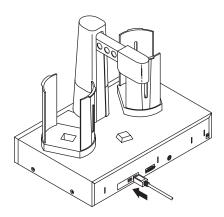
4. Connect the Serial Interface cable. One end is connected to the DB9 connector on the rear panel of the Duplicator. The other end is connected to your PC's DB9 COM1 port. If COM1 is already used for another device, you can use COM2 or COM3 and follow on-screen instructions later in the set-up procedure for changing the default serial port for the Duplicator.
