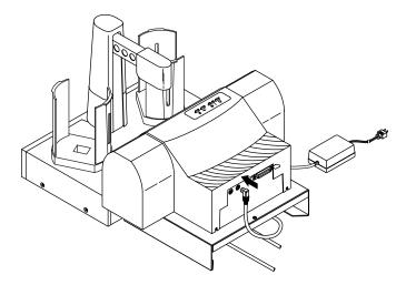
10. Connect the printer with an IEEE 1284 compliant parallel cable. One end is connected to the parallel port on the rear panel of the printer. The other end is connected to the parallel port of your PC. Make sure that your PC's parallel port is set to ECP mode. If you don't know how to check this or how to change it, refer to set-up section of the printer's Operator's Manual.
