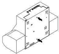
Position the printer on the stand so that the printer stand locating pins are inserted into the locating holes of the printer.
