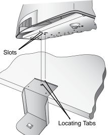
Place the Output Bin on the Output Bin Holder as shown.
