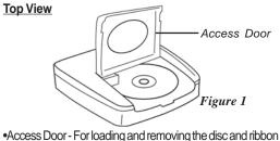
•Access Door - For loading and removing the disc and ribbon cartridge. (Refer to Figure 1)
