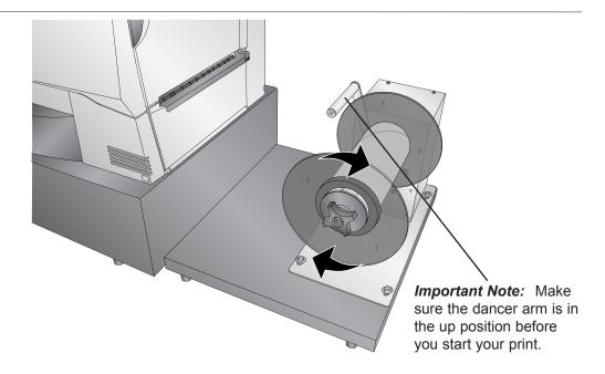
**Note:** Some cores may be shorter than the stock width. If so, make sure the distance between the label guide discs is slightly larger than the stock width.
