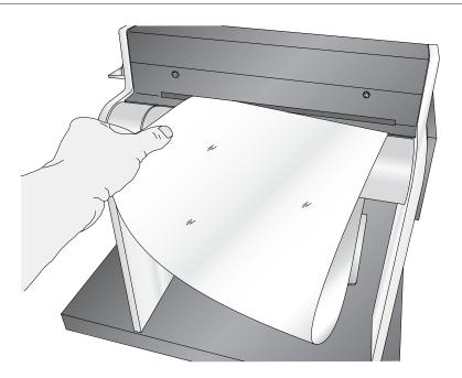
6. Continue feeding the stock into the printer feeder tray. Feed the stock under the sensor guard, under the green guides and under the paper feed roller. Stop feeding when the leading edge of the stock has covered the red stop block printed just outside the feeder door entrance.
