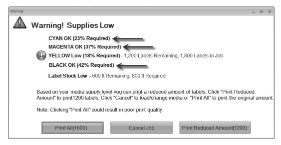
You will receive this warning if there is insufficient toner in any one of the four toner cartridges or if there is insufficient label stock on the supply roll. This calculation is based on the proof print that you must print before each job. The warning displays which cartridges are low on toner for this job and the percentage of toner from each cartridge that is required. You have several options at this point.
