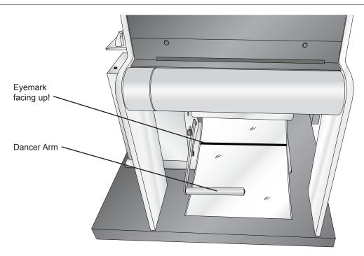
5. Continue feeding the stock over the roller and through the cutter. Feed the stock throught the cutter at an angle.
