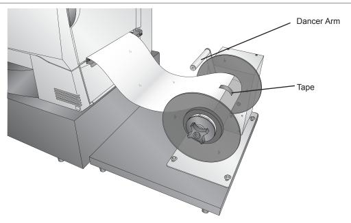
11. Immediately after the label stock is attached, engage the Rewinder by flipping the Rewinder Dancer Arm toward the printer until it touches the paper.
