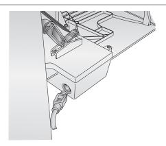
20. Connect the other end of this cable to the connector port on the right side or farthest away from the printer.
