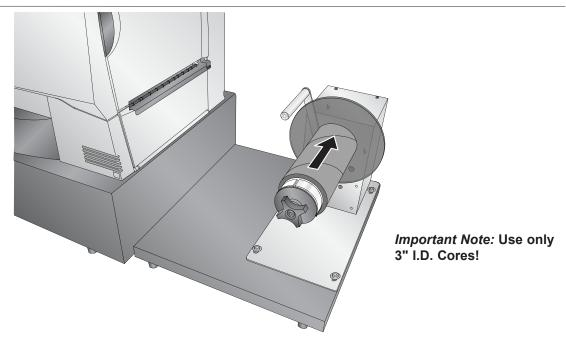
8. Place the outer label guide disc on to the rewinder chuck. Push the guide until it touches the rewinder core. Turn the tension knob clockwise to secure the core and the label guide to the chuck.
