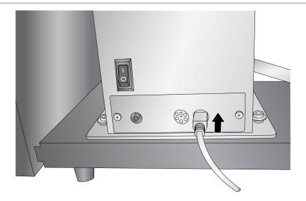
21. Connect the remaining 6-pin round cable to the back of the cutter mechanism and to the remaining port on the unwinder closest to the printer.
