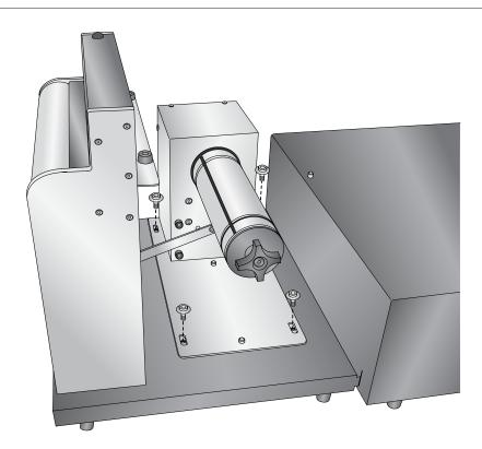
9. Locate the rewinder stand. Attach it to the right side of the printer base. Align the hooks on the rewinder stand to the slots on the printer stand.
