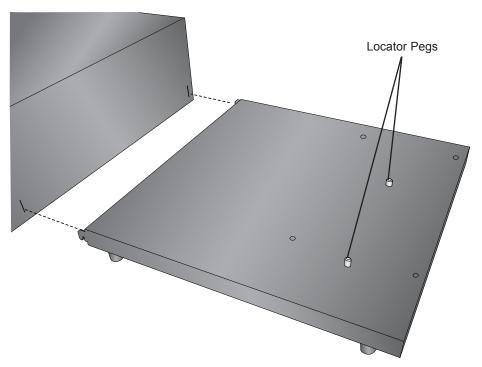
10. Locate the rewinder. The rewinder has a longer dancer arm and no 6-pin ports on the back. Attach it to the stand using the #2 Phillips screws and the washers found in the hardware bag. Use the locator pegs on the stand and align them with the holes on the bottom of the rewinder.
