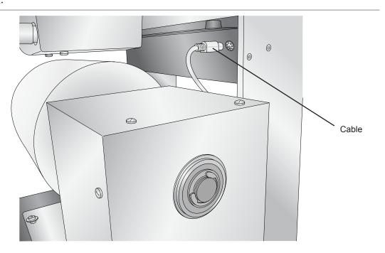
22. Locate the power converters and the printer power cord. Connect power to the printer and switch on the power. Connect the power to the back of the rewinder and unwinder. Switch on the power.
