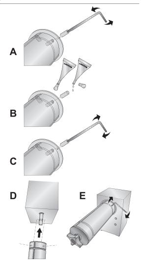
5. Locate the rewinder (right side) chuck, the label guide disc with the three interior holes, the rewinder, the loctite and the 3mm allen wrench. The rewinder has a longer dancer arm and no 6-pin ports on the back.
