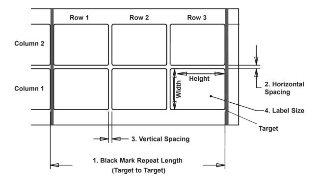
**Note:** Targets are printed on the back of the label stock liner.
