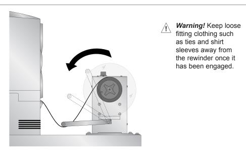
**Important!** To minimize the slack loop that will be created under the rewinder, it is very important that you lower the dancer arm immediately after the label stock is taped to the core.
