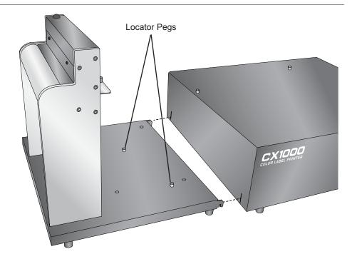
Locate the unwinder. It has the shorter dancer arm and two 6-pin ports on the back. Attach it to the stand using the #2 Phillips screws and the washers found in the hardware bag. Use the locator pegs on the stand and align them with the holes on the bottom of the unwinder.
