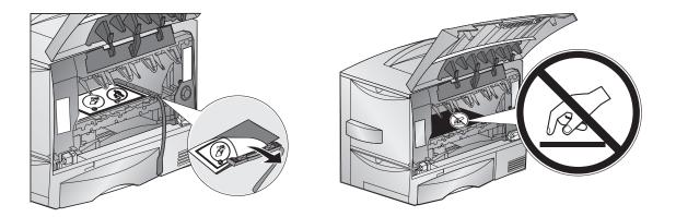
16. Before replacing the toner cartridges remove the red plastic protection plate from the bottom of each toner cartridge. Put cartridges back in to the printer. On each cartridge there are pegs that correspond to slide rails inside the printer.
