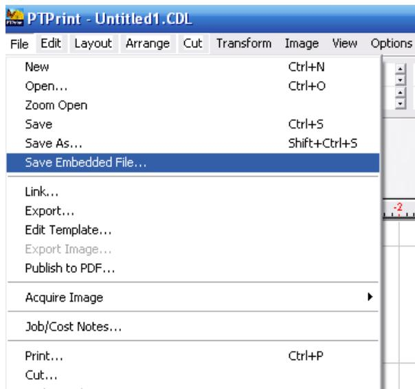
**3 .** Finally, create a cut file. Save it with each CDL file. Name the cut file the same as the CDL file except the plt extension which is automatically added. If you ever move them to a new location, keep the cut file with the print file.
