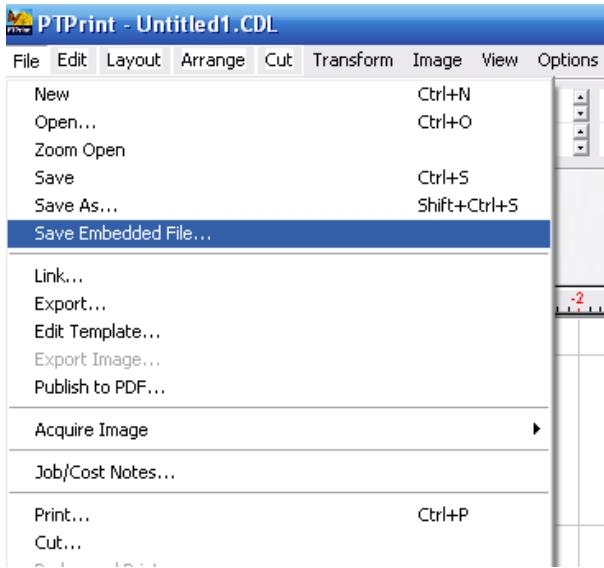
**4. Finally, create a cut file. (Skip this step if printing to a CX100) Save it with the CDL file. You will use this cut file for all of the labels in the batch when you cut them on the FX1200.**
