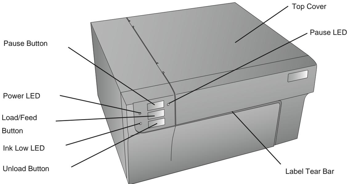
The **Pause Button** is pressed to pause a job to allow for loading of label stock and ink cartridges. The Printer pauses after the printing of the current label has finished. The Pause LED will illuminate when the Printer is paused.
