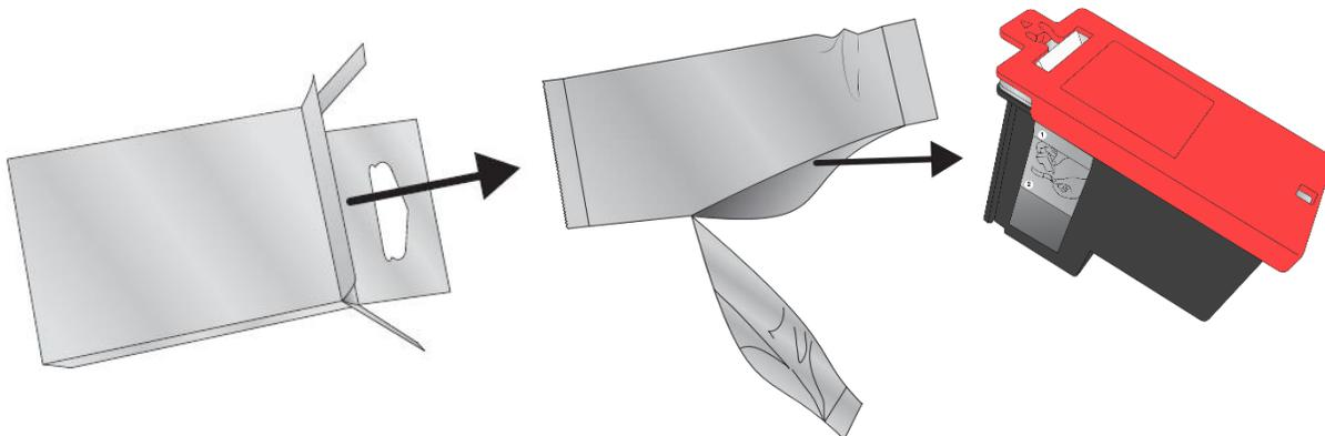
5. Remove and discard the red protection cap and peel off the tape covering the nozzle.
