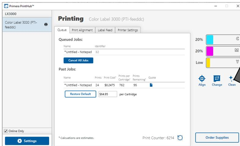
2. Determine if printing is now acceptable by printing your image. If the sample has missing colors or voids within a color strip, remove the cartridge from the printer and proceed to step 4.
