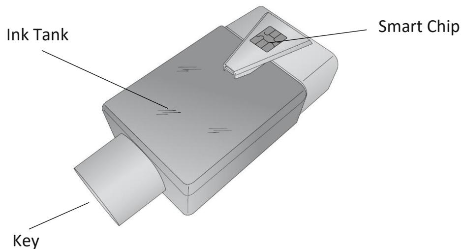
3. Match the ink tank color with the sticker behind the corresponding slot on inside the Printer. Hook the chip to the slot.
