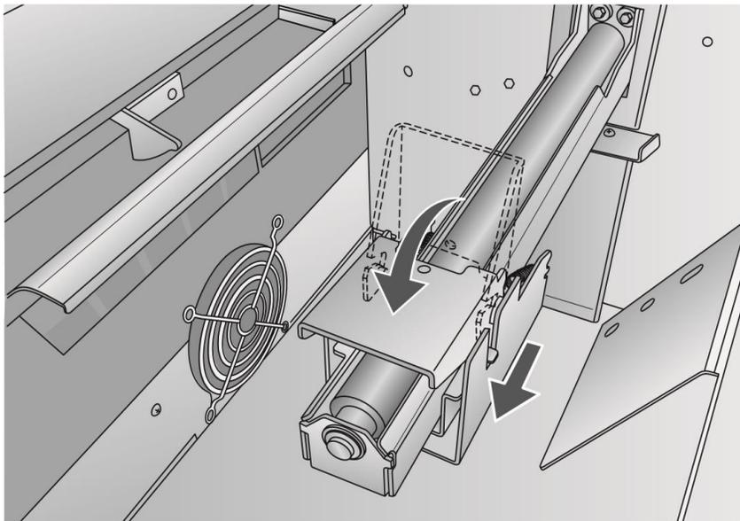
3. Remove any shipping tape from your label stock roll to ensure that it can unroll freely, making certain that no adhesive portion is exposed. It is important to note that any exposed adhesive surface can attach itself to the inner workings of the print mechanism and cause a media jam.
