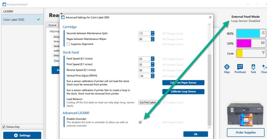
**Tip:** Leave a roll of labels installed on the internal unwinder so that your external labels will feed more easily past the roll bar.
