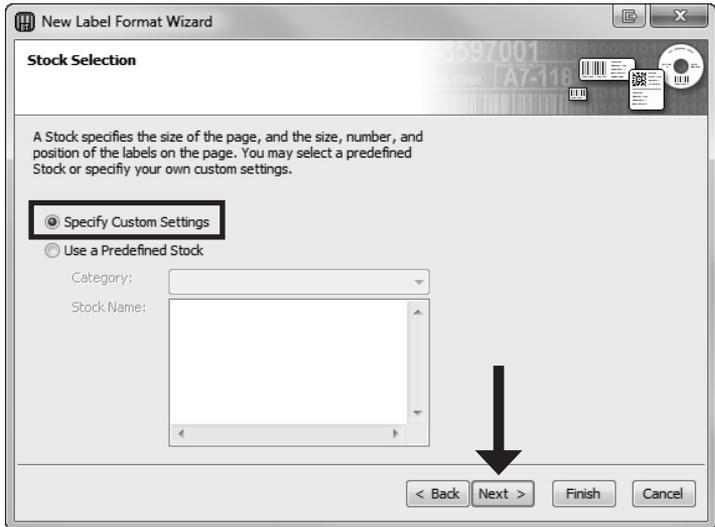
5. Set the page size, width and height to match labels installed in the printer. Click "Next".
