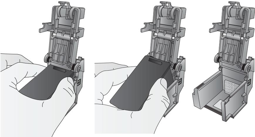
4. Locate a new cartridge and remove it from its packaging. Remove the foil outer package and the tape covering the nozzles.
