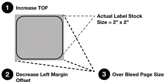
**Note:** *It is best to over bleed as little as possible to avoid excess ink on the label backing. Also, over bleeding too much will cause the printer to skip labels. This is because the printer stops printing too late to sense the next label.*
