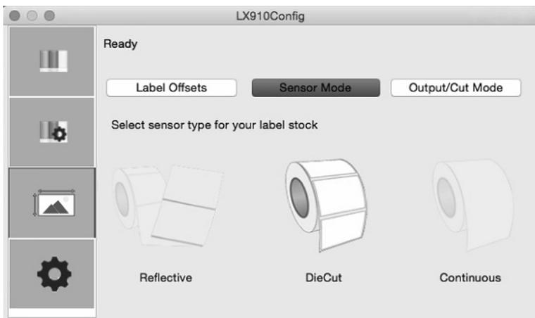
**Important Note:** Set the Stock Sensor Mode *BEFORE* loading label stock! You must also set the Stock Sensor Position (Section 2C) so that the sensor is sensing the correct point on the label stock.
