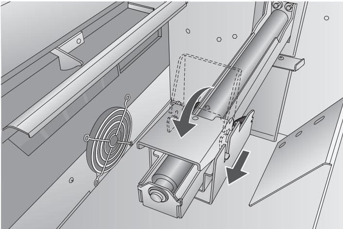
3. Remove any shipping tape from your label stock roll to ensure that it can unroll freely, making certain that no adhesive portion is exposed. It is important to note that any exposed adhesive surface can attach itself to the inner workings of the print mechanism and cause a media jam.
