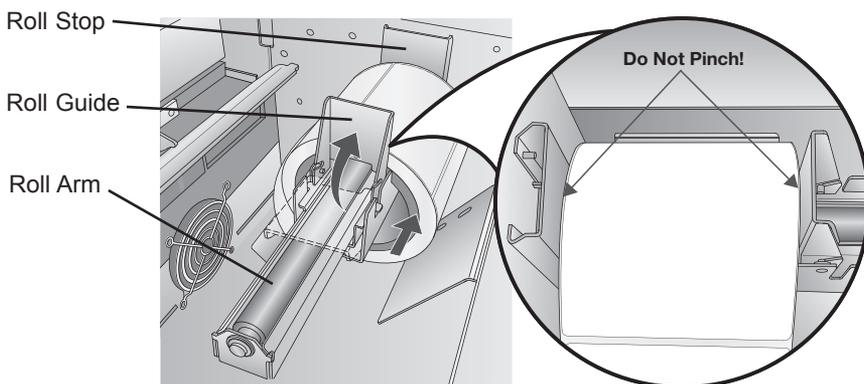
5. Flip up the Roll Guide and slide it inward until it touches the label stock. The Roll Guide will automatically pull back slightly to the correct position. There should be approximately a 1mm gap between the Roll Guide and the roll.
