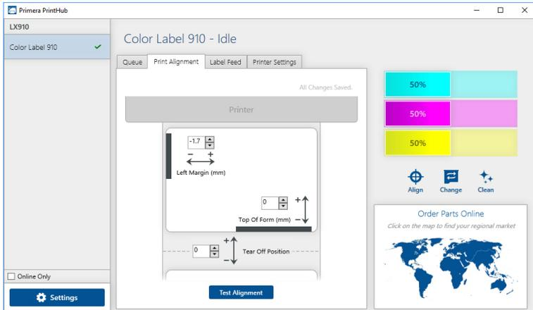
**Important!** Before adjusting any values, print the Test print to see how close you are to alignment. The on screen graphic is the same as the print which makes it easier to adjust these values.
