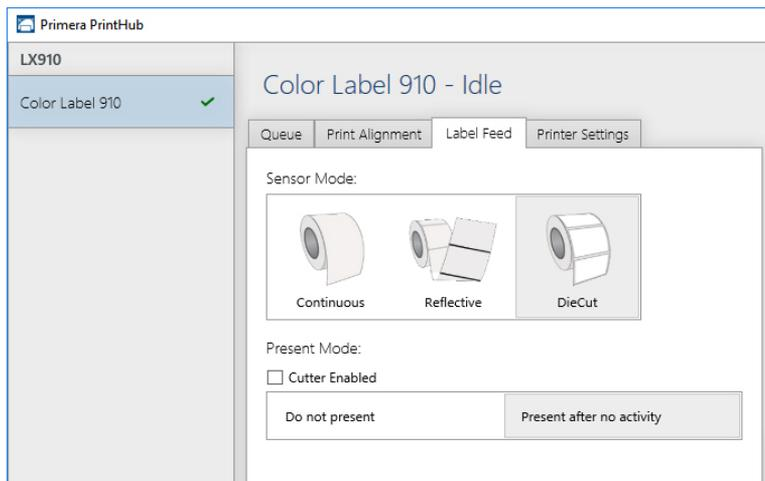
**Do not present.** In this mode the label stock does not move after the last label is printed. This means that part of the last label printed is still in the printer. This should be used only if you have a label rewinder attached.
