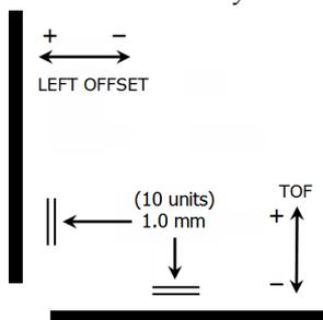
You may have to make several adjustments to one or more of these values. After each adjustment you can click the Test button to print a small test pattern on the label. This will help you find the proper alignment value.
