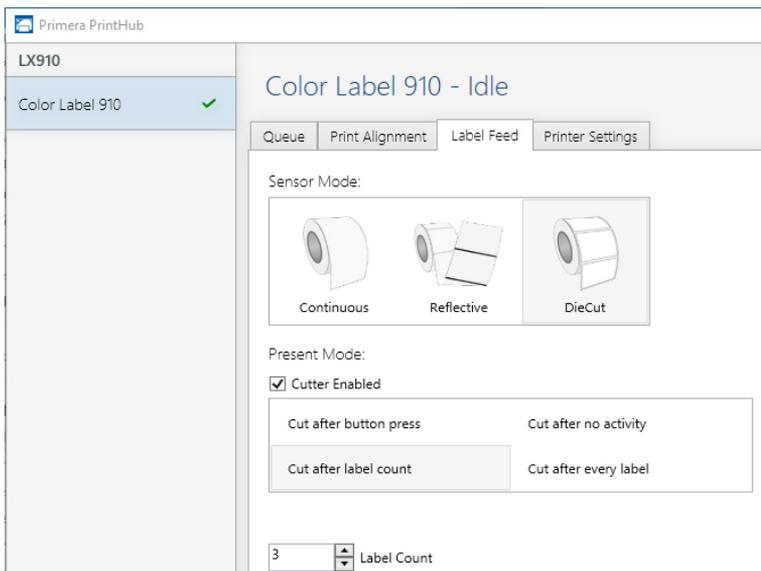
**Cut after button press.** This setting will cut after you press the Load/Feed button on the printer. This can be used after one label or an entire job. This feature is useful if you will not be present at the end of the print to catch the cut label.
