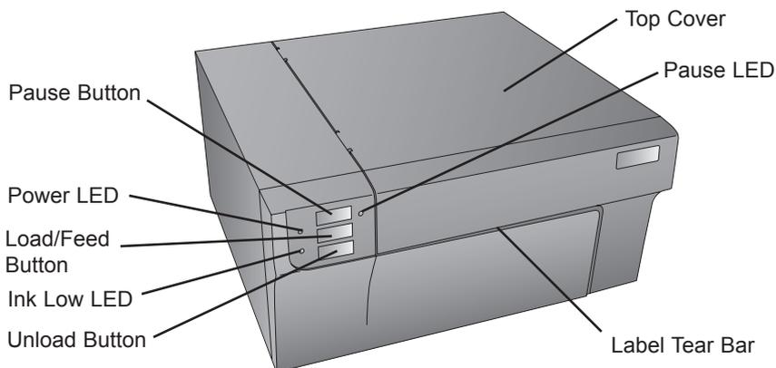
The **Pause Button** is pressed to pause a job to allow for loading of label stock and ink cartridges. The printer pauses after the printing of the current label has finished. The Pause LED will illuminate when the printer is paused.
