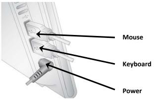
**1.** Connect the keyboard, mouse and power connector to the <u>left side</u> of the touch screen computer.
