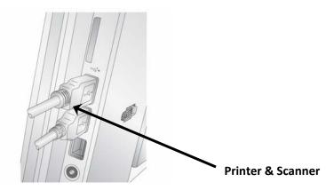
**2.** Connect the USB cable for the Slide Printer to <u>right side</u> of the touch screen computer and the back of the printer. Connect the Scanner (optional) to the right side of the computer.
